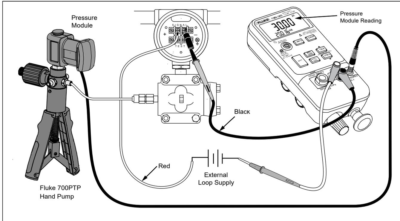
Figure 5. Pressure Module with External Pump
