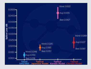
Maximum allowed splice loss for installations that comply with ISO/EN/TIA standards is 0.30dB. FiberMASTER splice loss exceeds these standards by more than 20x, reducing attenuation in your fibre links and increasing overall system margin. Data from 100 splices measured with laboratory test equipment. Not the loss displayed on the fusion splicer screen.
